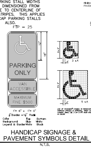
HANDICAP SIGNAGE & PAVEMENT SYMBOLS DETAIL N.T.S.
