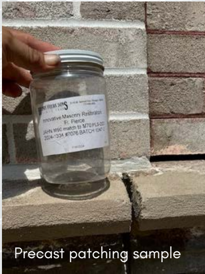
Custom formulated mixes for patching samples of the precast and foundation
