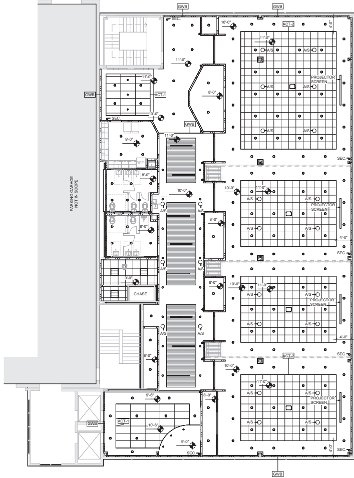
1 4TH FLOOR REFLECTED CEILING PLAN SCALE: 1/8" = 1'-0"
