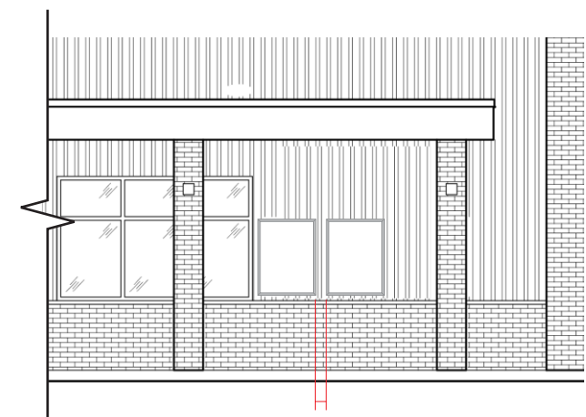
ELEVATION: WALK-UP WINDOW SCALE: 1/8"=1'-0" (UNLESS OTHERWISE DIRECTED) 2" INSET FROM MULLION 2" ABOVE STONE CAP 6" BETWEEN MENUS
