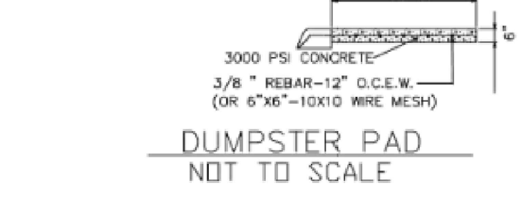
D DUMPSTER PAD STALL DETAIL SCALE: NONE
