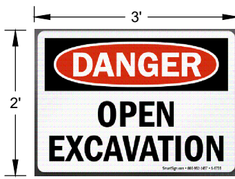
EXCAVATION WARNING SIGN DETAIL N.T.S.
