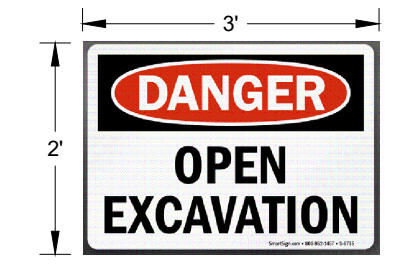
EXCAVATION WARNING SIGN DETAIL N.T.S.
