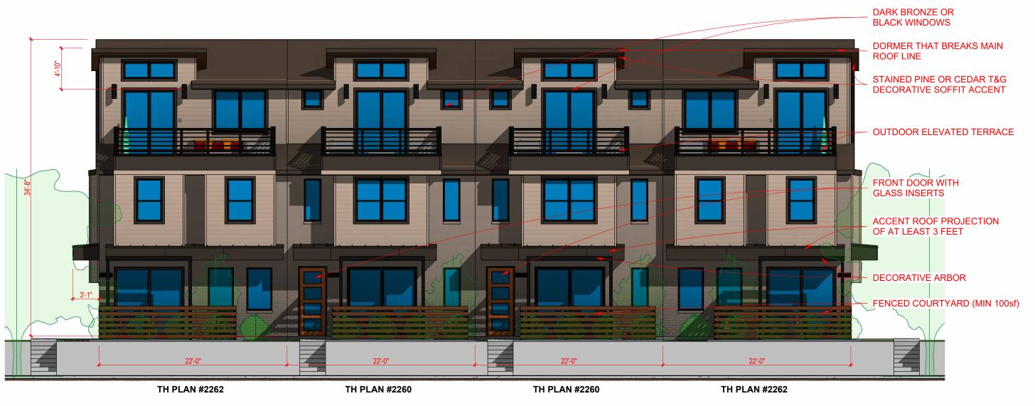
**BUILDING SIDE ELEVATION & CROSS-SECTION** 1/8" = 1'-0"
