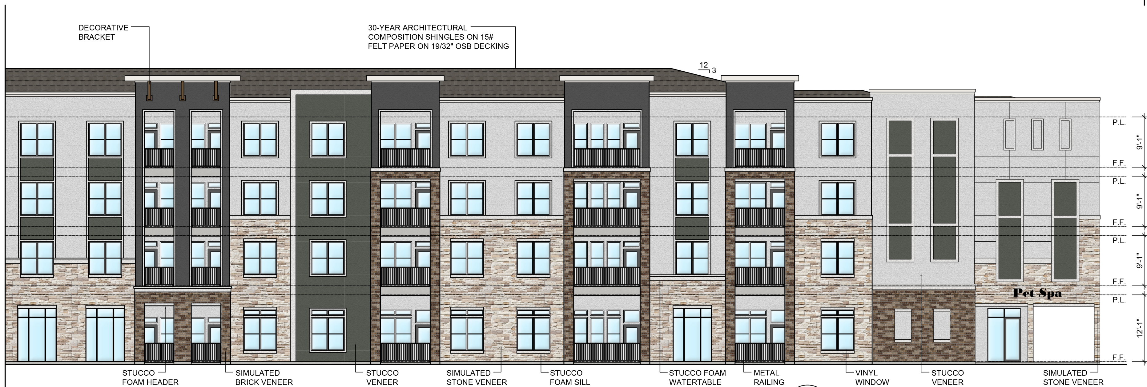
01 BUILDING 'E' - REAR ELEVATION SCALE: 3/32" = 1'-0"
