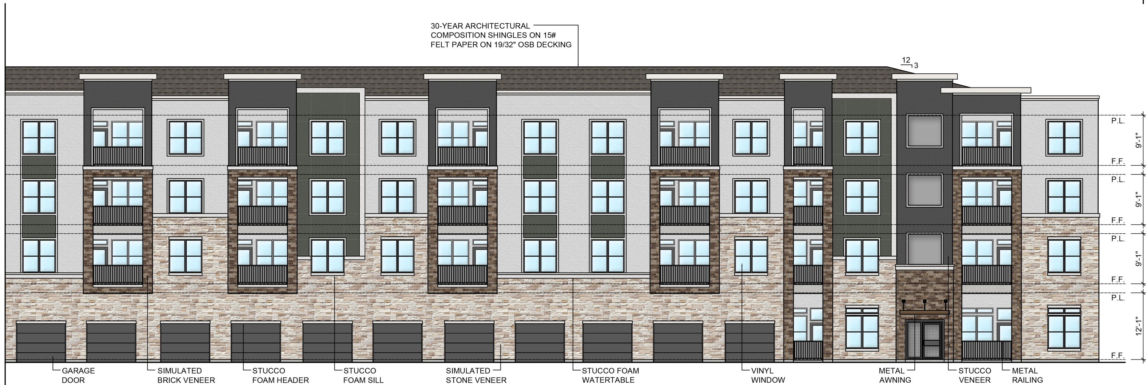
01 BUILDING 'E' - FRONT ELEVATION SCALE: 3/32" = 1'-0"
