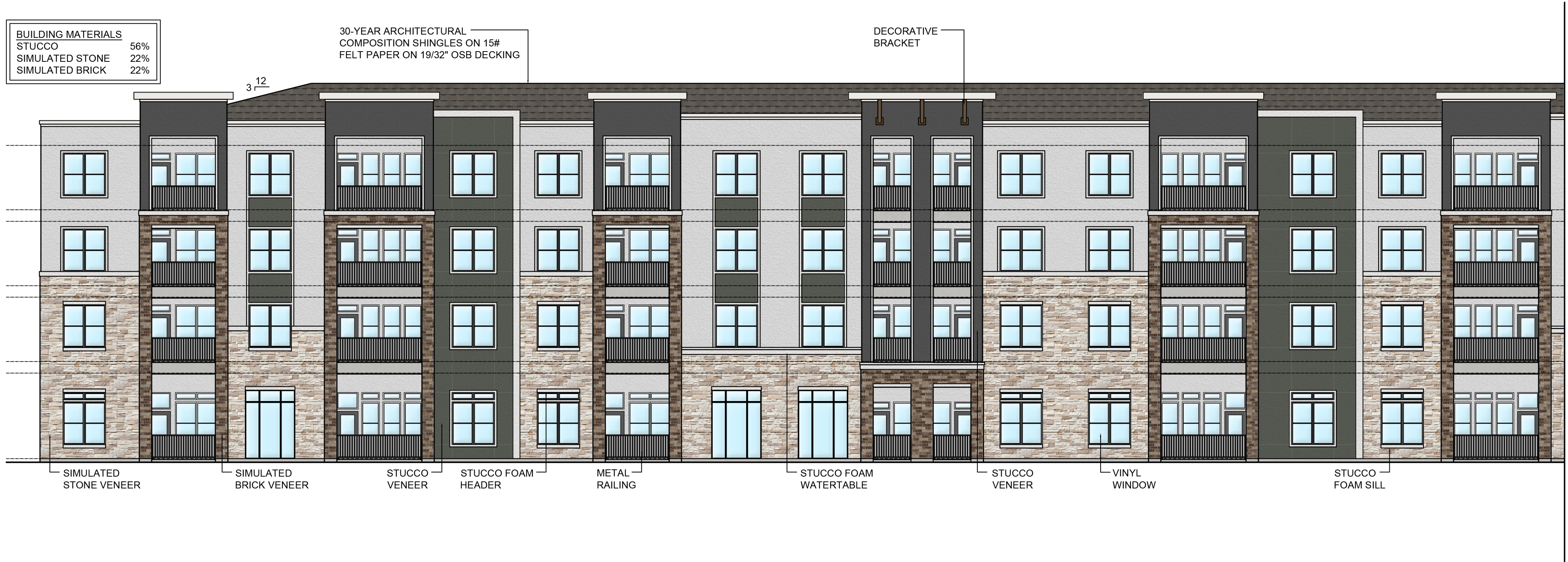
02 BUILDING 'E' - LEFT ELEVATION SCALE: 3/32" = 1'-0"
