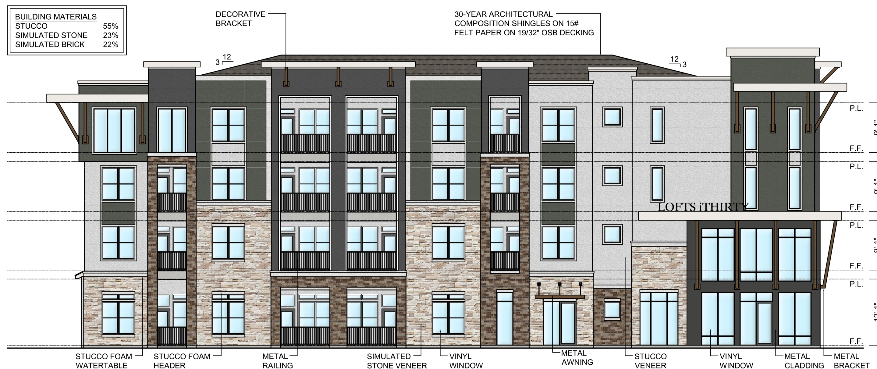
01 BUILDING 'A' - FRONT ELEVATION SCALE: 3/32" = 1'-0"
