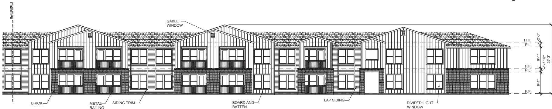
BUILDING 'B' EAST ELEVATION
