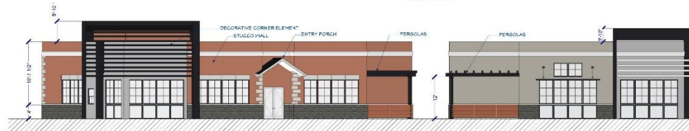
WEST ELEVATION - BUILDING #2 & #3 SCALE - 1/8" = 1'-0"
