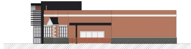
SOUTH ELEVATION - BUILDING #3 SCALE - 1/8" = 1'-0"
