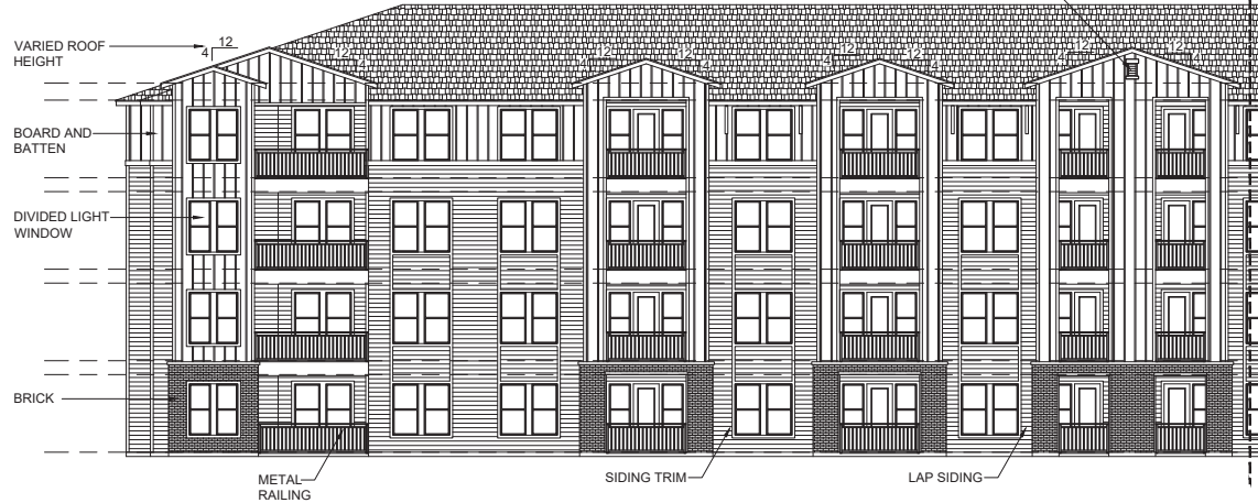
BUILDING 'A' SOUTH ELEVATION
