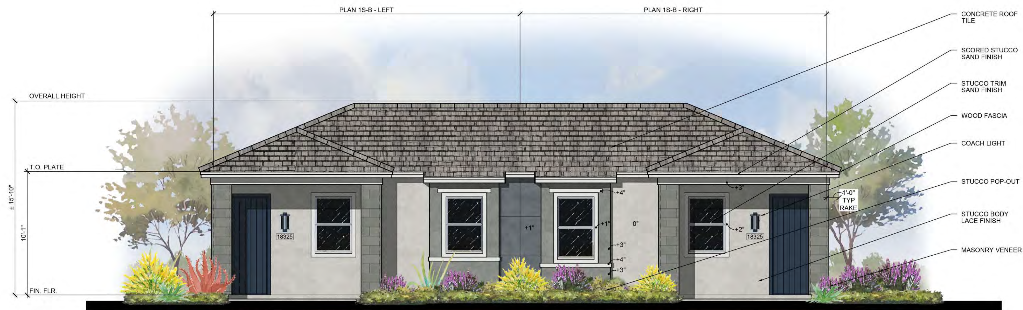
FRONT ELEVATION Elevation B - Desert Contemporary 1/4" = 1'-0"
