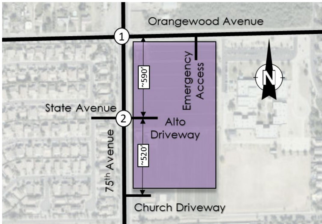
Figure 6: Existing Driveway Access Spacing
