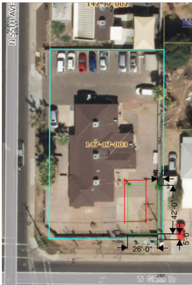
Image 1. Available shaded area per UDC shown in red; proposed shaded area in green.
