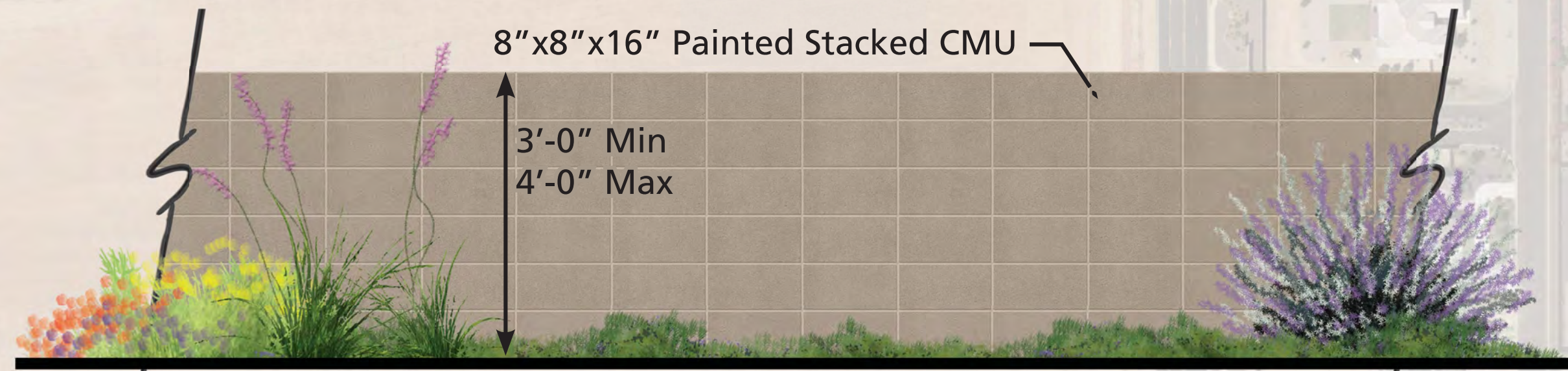
TYPICAL PARKING SCREEN WALL
