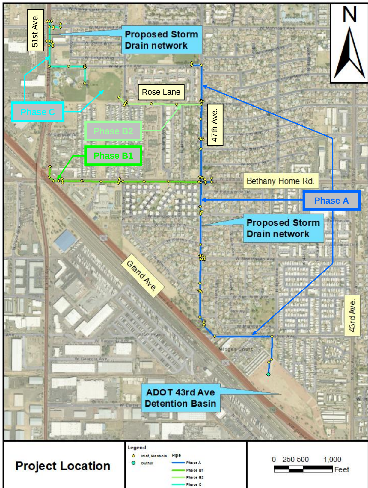
Figure 1: Project Proposed Storm Drain Improvements
