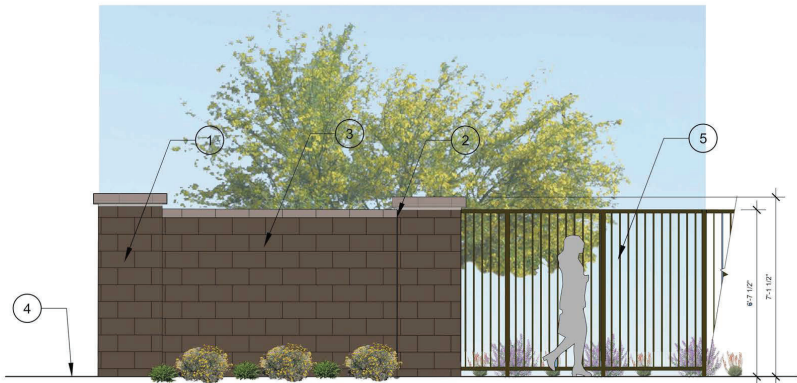
A ENHANCED COMMUNITY PERIMETER WALL SCALE: 1/2" = 1'-0"
