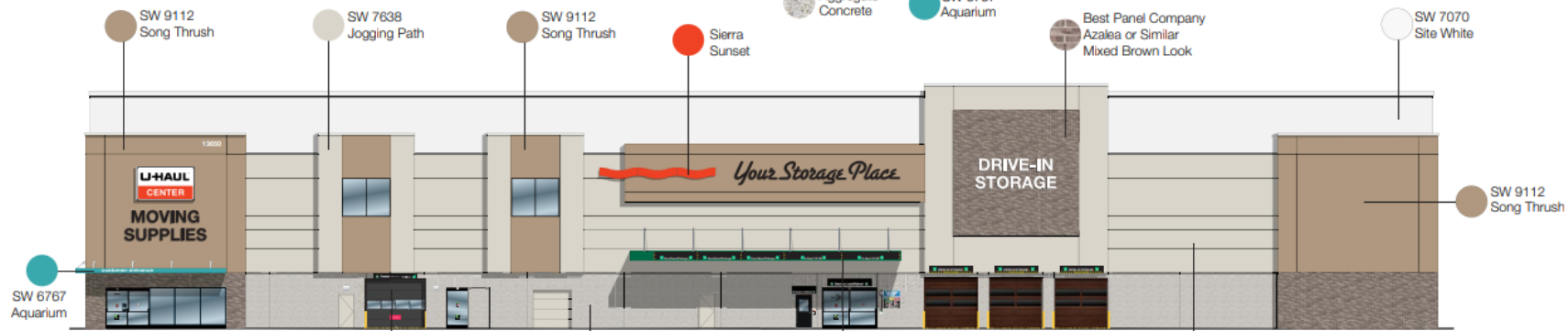
NORTH ELEVATION - BLDG. A Scale: 1" = 20'
