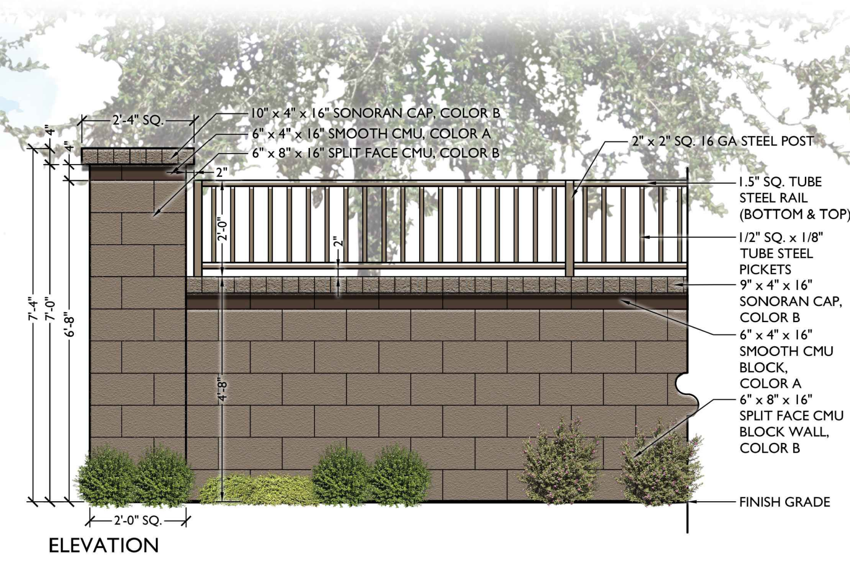
3 PARTIAL VIEW WALL - TYPE 2 Scale: 1/2" = 1'-0"
