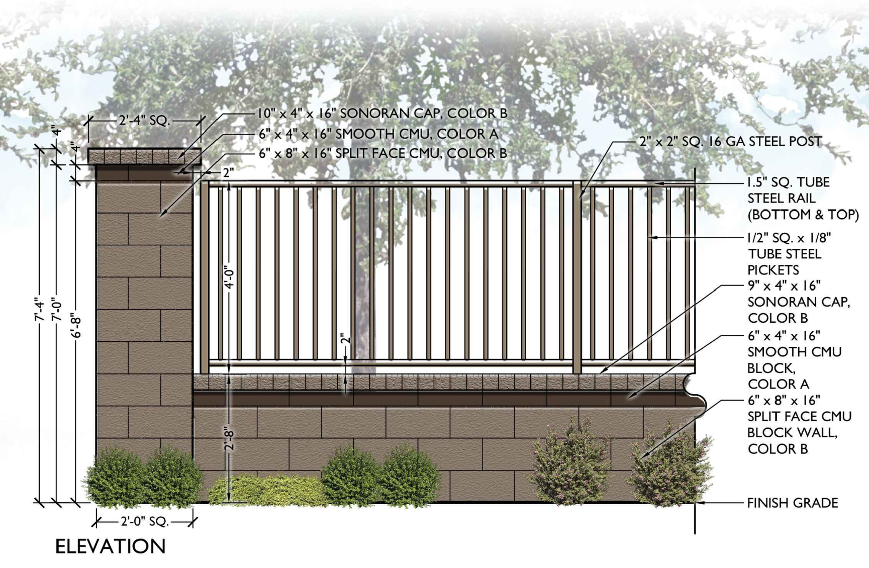
2 PARTIAL VIEW WALL - TYPE 1 Scale: 1/2" = 1'-0"
