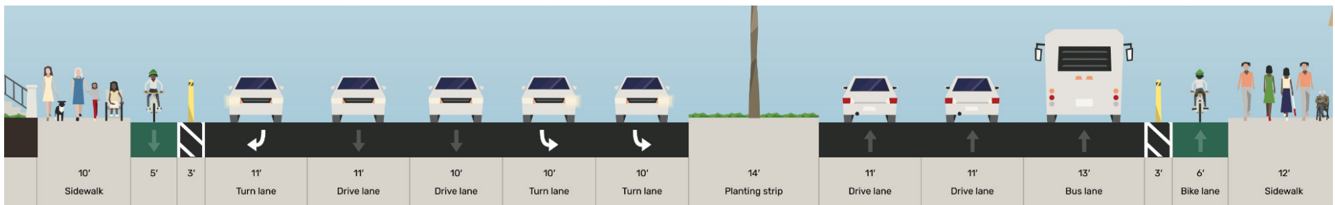
Exhibit 19. Proposed cross-section: Hawthorne Boulevard from north City limits to Imperial Hwy
