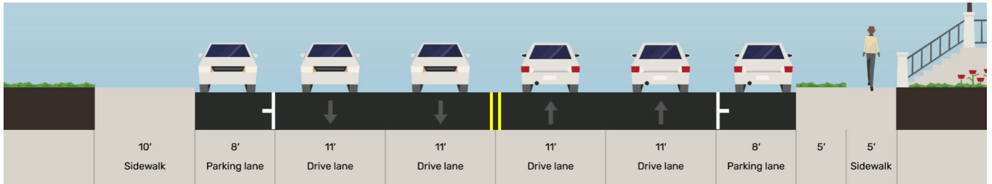
Exhibit 51. Existing cross-section: W 135 th St from Aviation Blvd to La Cienega Blvd
