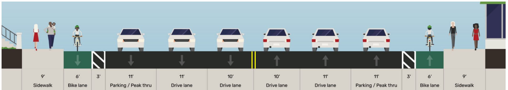
Exhibit 30. Proposed cross-section: El Segundo Blvd from Aviation Blvd to east city limits
