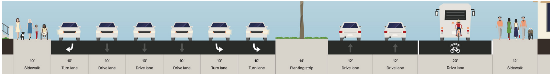
Exhibit 18. Existing cross-section: Hawthorne Boulevard from north City limits to Imperial Hwy
