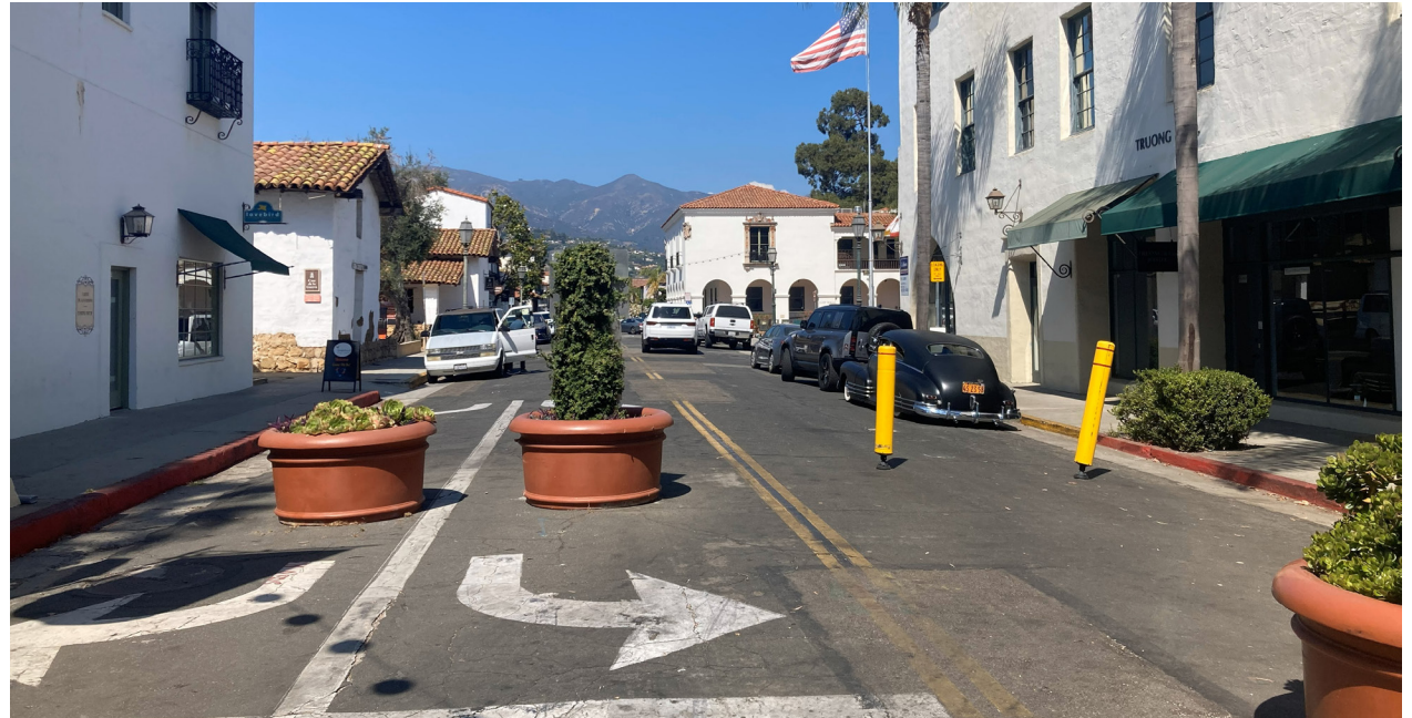
Exhibit 81. Temporary modal filter with flex posts, preserving emergency access, in Santa Barbara, CA
