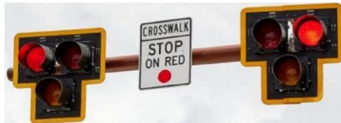
Figure 4: Pedestrian Hybrid Beacon
