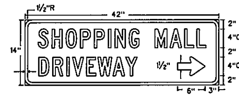
D-70S 42" X 14" Letters - White Refl. Symbol - White Refl. Border - White Refl. Background - Blue Refl.
