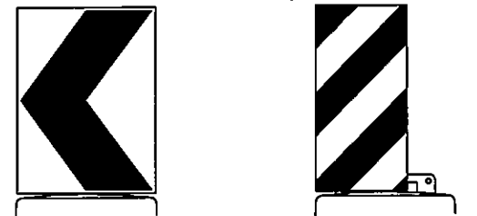
18" x 24" Sign (Maximum Sign Dimension) Chevron CW1-8, Driveway sign D70a, Keep Right R4 series or other signs as approved by Engineer
