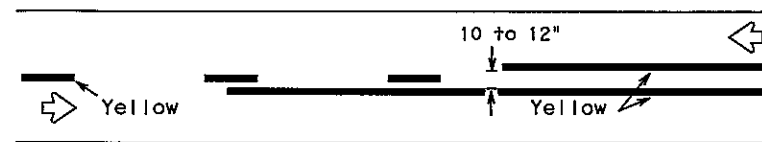
REFLECTORIZED PAVEMENT MARKINGS - PATTERN A
