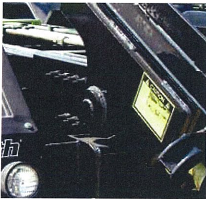
Hoist frame huck bolted to chassis on all factory mounted hoists
