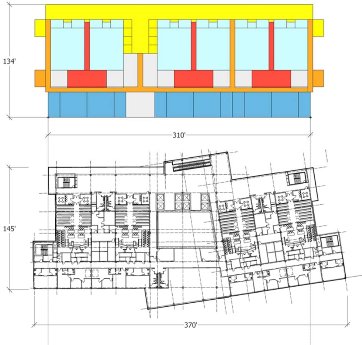
Illustration of 6 Courts per floor in the same footprint as 4 court per floor
