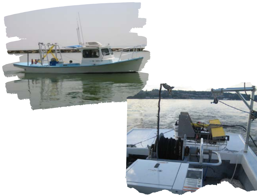
Figure B1: Research vessel (left) and Tow-body (right) carry instrument suite
