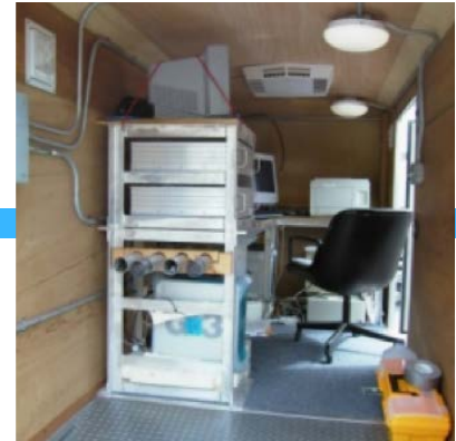
Left to right: a) HF-radar antenna (left) b) Mobile HF-radar unit (Center) & c) Inside of mobile unit (right) which contains the data acquisition and processing system along with other necessary components.
