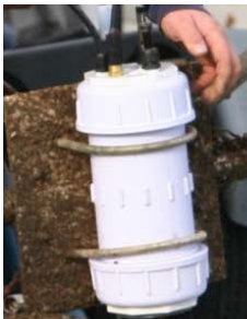
Figure A4 Replacement of prototype standard water quality sonde at field testing node located near Wappingers
