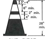
ONE-PIECE PLASTIC CONE (28" MIN. HEIGHT) 3
