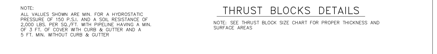
W-5 THRUST BLOCKS DETAILS
