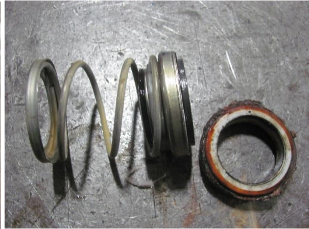
Mech Seal Worn
