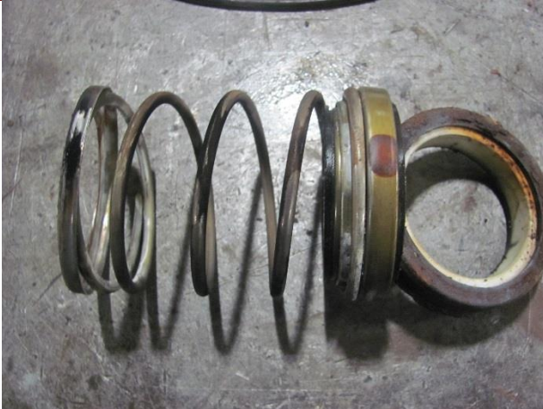
Mech Seal Worn
