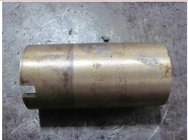
Shaft Sleeve Worn
