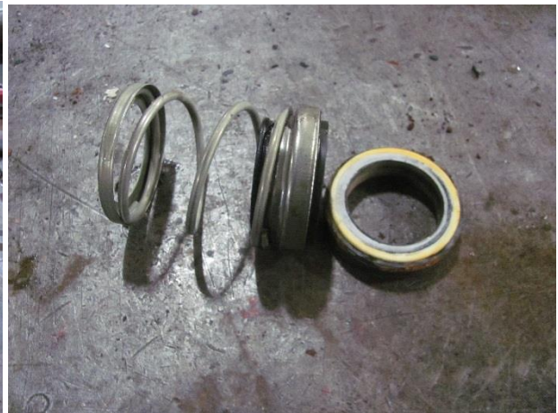
Mech Seal Worn
