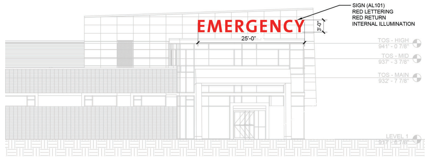
Example EMERGENCY signage (QTY 2) Would be installed on both sides of building element 75 SF x 2 = 150 SF Cap Height 3'-0" Font: The Sans B7 Bold
