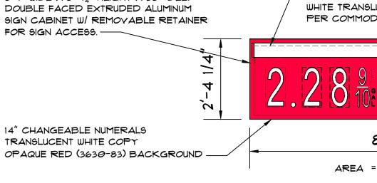
8'-1" WIDE  $\times$  2'-4 $\frac{1}{4}$ " HEIGHT  $\times$  20" DEEP DOUBLE FACED EXTRUDED ALUMINUM SIGN CABINET W/ REMOVABLE RETAINER
