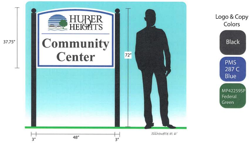
Furnish and install (1) double faced non-illuminated post and panel sign. Overall size of top panel 37.75 "H x 48"W totaling 12.58 square feet. Panel to be 3/4 routed PVC with aluminum frame kit. Panel face routed out to create raised copy, and graphics and border. Face decorated with first surface paint (PMS 287 & MP42259SP Federal Green & Black) Post are 3" round aluminum Painted Black with 3" round tops Painted Black.
