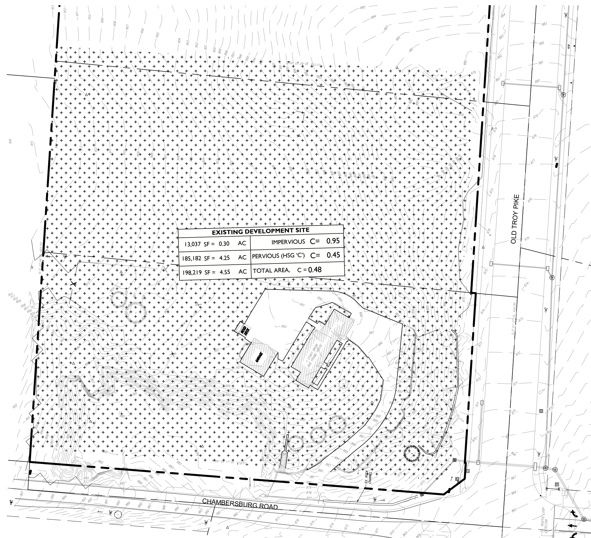
EXISTING SITE COVERAGE GRAPHIC SCALE IN FEET 1" = 60'
