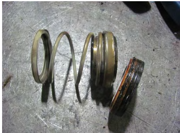
Mech Seal Worn
