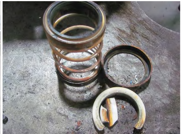
Mech Seal Worn
