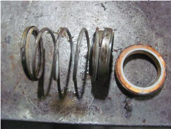
Mech Seal Worn
