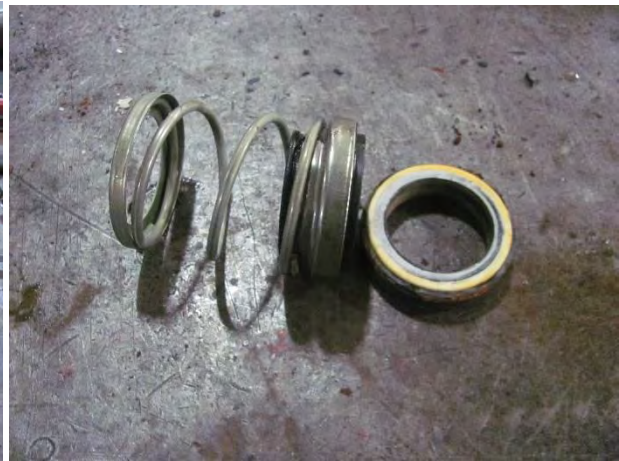
Mech Seal Worn
