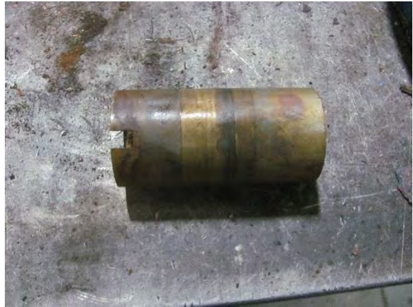
Shaft Sleeve Worn
