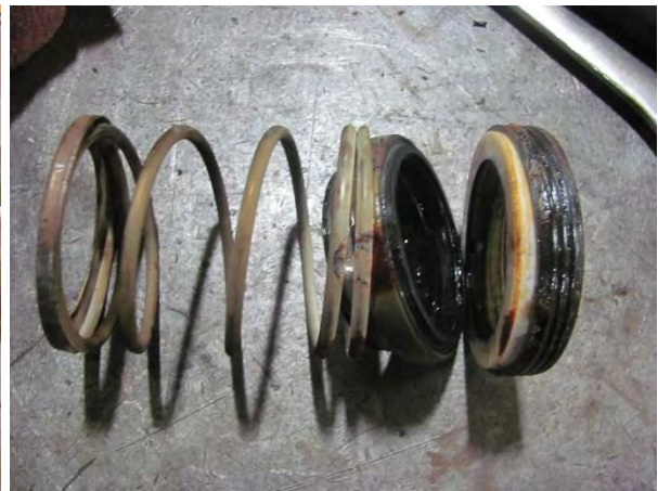
Mech Seal Worn
