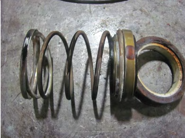
Mech Seal Worn
