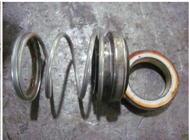
Mech Seal Worn
