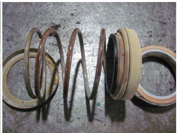
Mech Seal Worn
