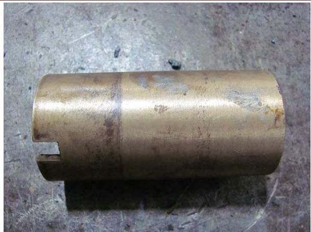
Shaft Sleeve Worn
