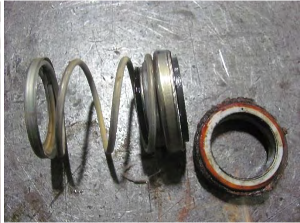
Mech Seal Worn
