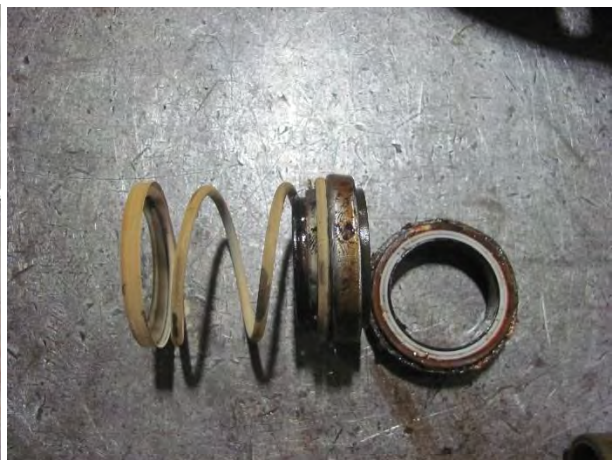
Mech Seal Worn
