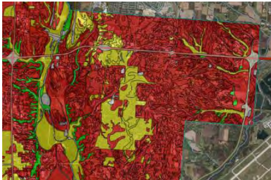
Figure 3-15. Risk of Soil Corrosion for Steel (Montgomery County only) (Yellow = Moderate Corrosivity for Steel; Red = High Corrosivity for Steel)
