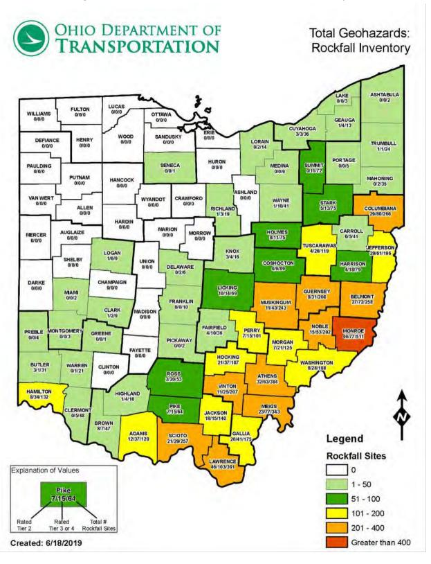
Figure 4.6.6: State of Ohio Total Geohazards Rockfall Inventory
