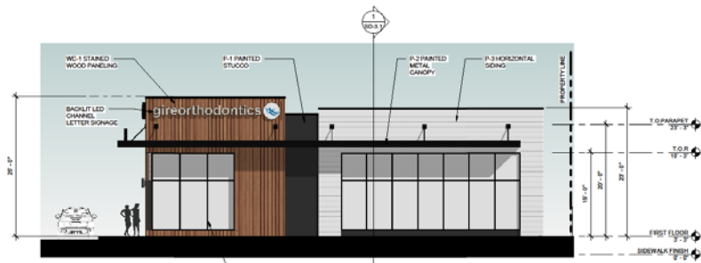
SOUTH ELEVATION - STREET VIEW 3 1/8" = 1'-0"
