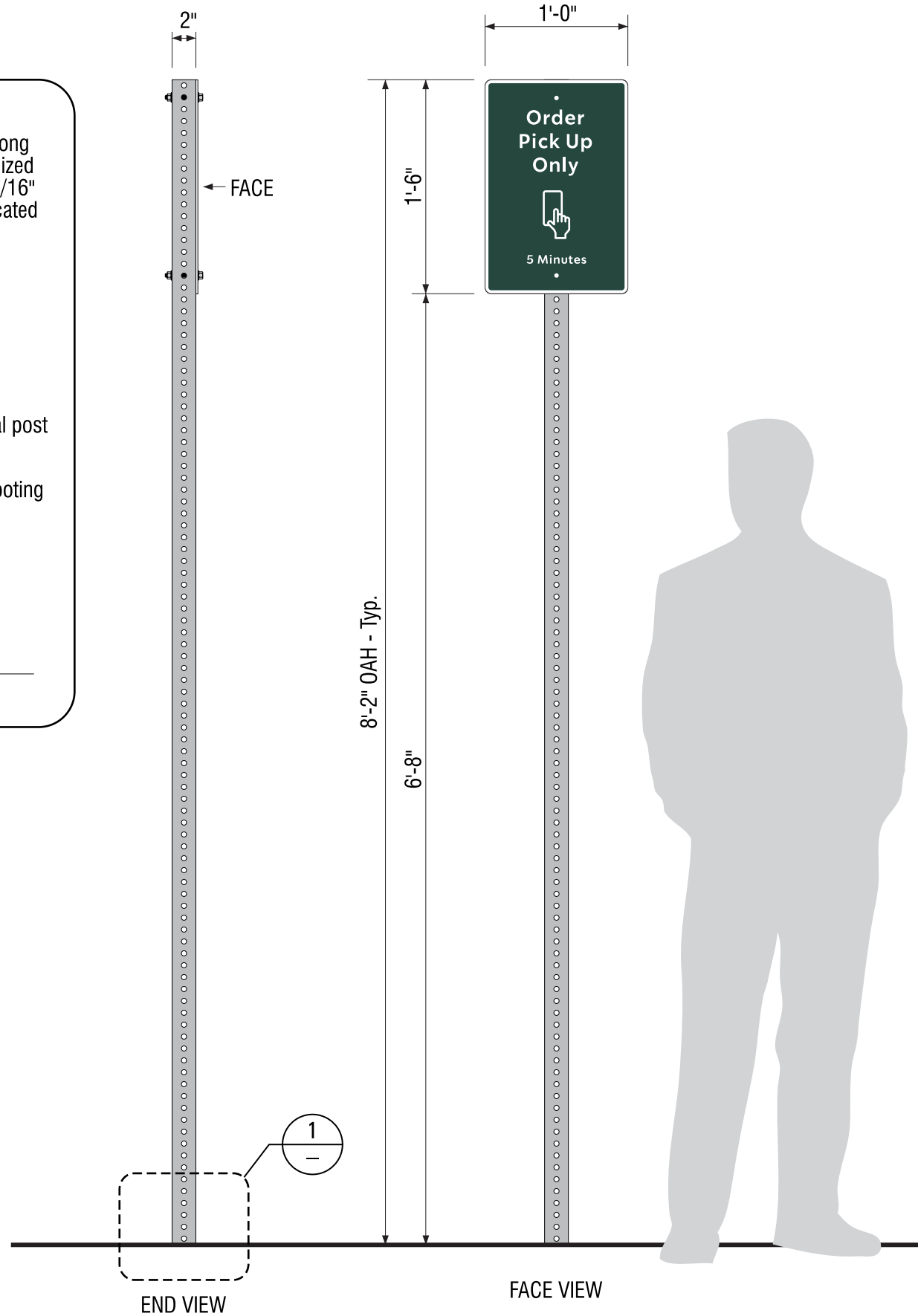
NEW S/F "MOP 5 MINUTE PARKING" POST & PANEL SIGN - TYPICAL SIGN AREA: 1.5 Sq. Ft.
