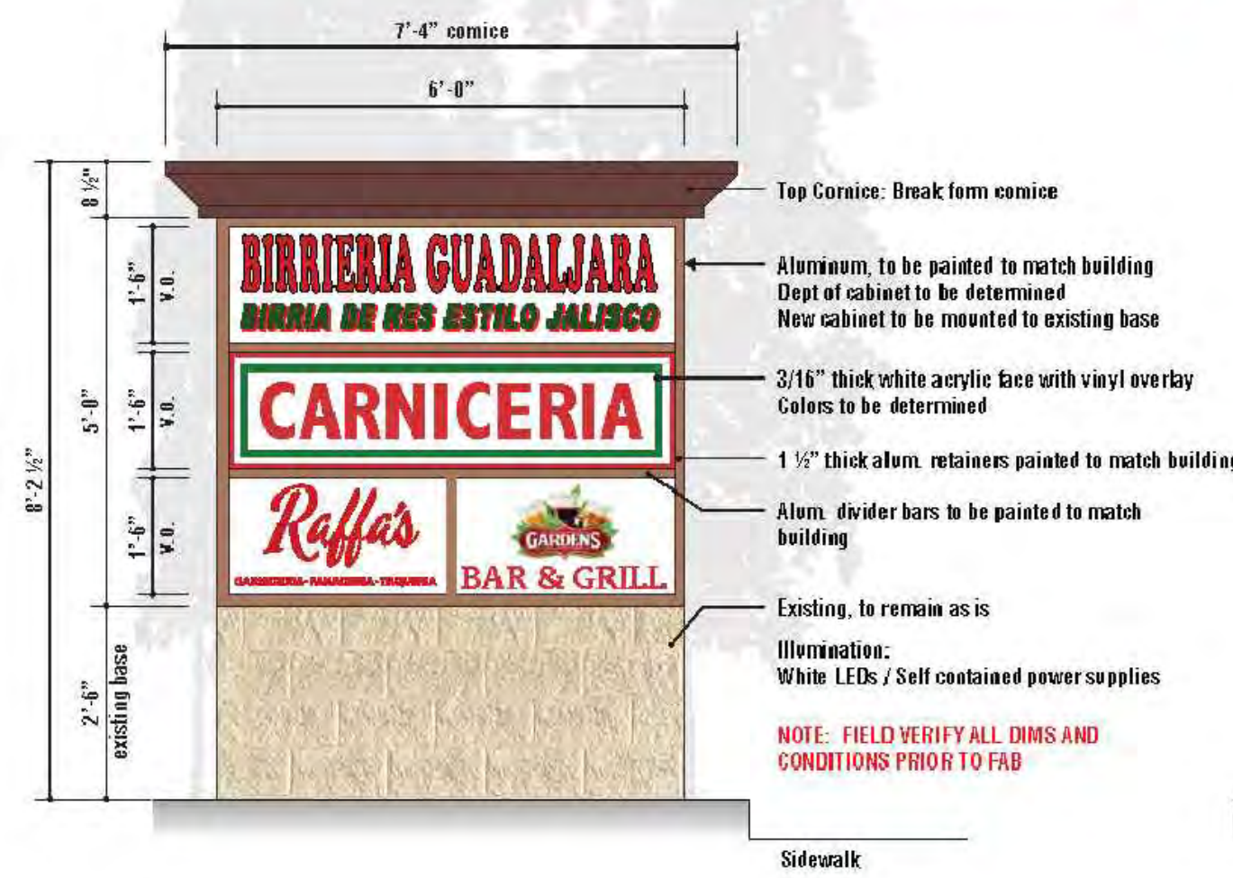
N Front View - La Habra Blvd City: One (1) Square Footage: 30 Scale: 1/2" = 1'-0" Refurbish existing double face illuminated monument sign Manufacture and install new double face illuminated cabinet
