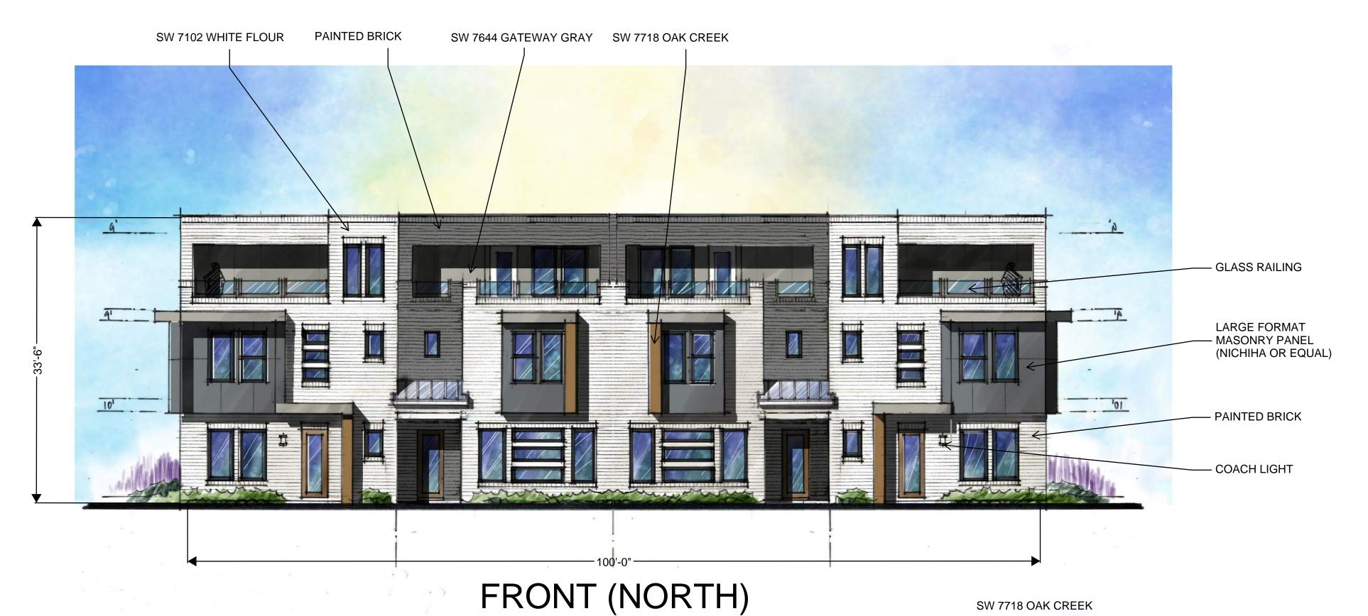
FRONT (NORTH) FACADE: TOTAL MATERIAL SURFACE AREA = 2676 SQ. FT. MASONRY PANEL: 794 SQ. FT. = 24.74% PAINTED BRICK: 2014 SQ. FT. = 75.26%
