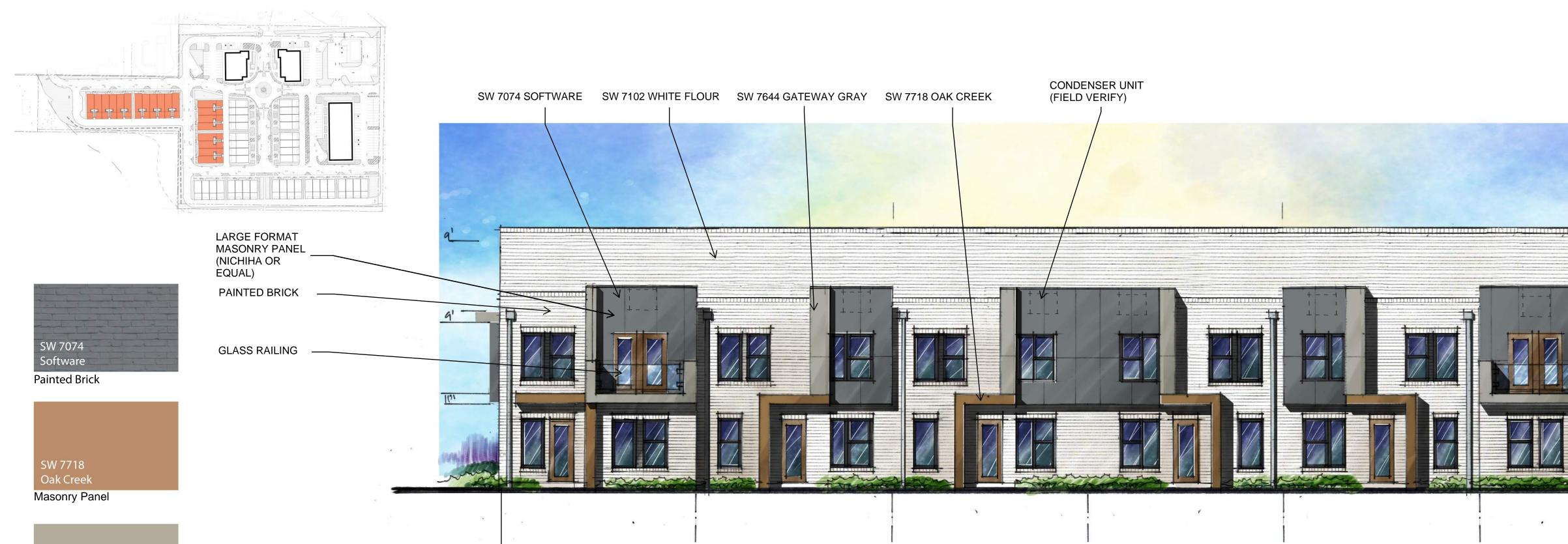
FRONT (WEST) FACADE: TOTAL MATERIAL SURFACE AREA = 4100 SQ. FT. MASONRY PANEL: 1024 SQ. FT. = 24.98% PAINTED BRICK: 3076 SQ. FT. = 75.02%
