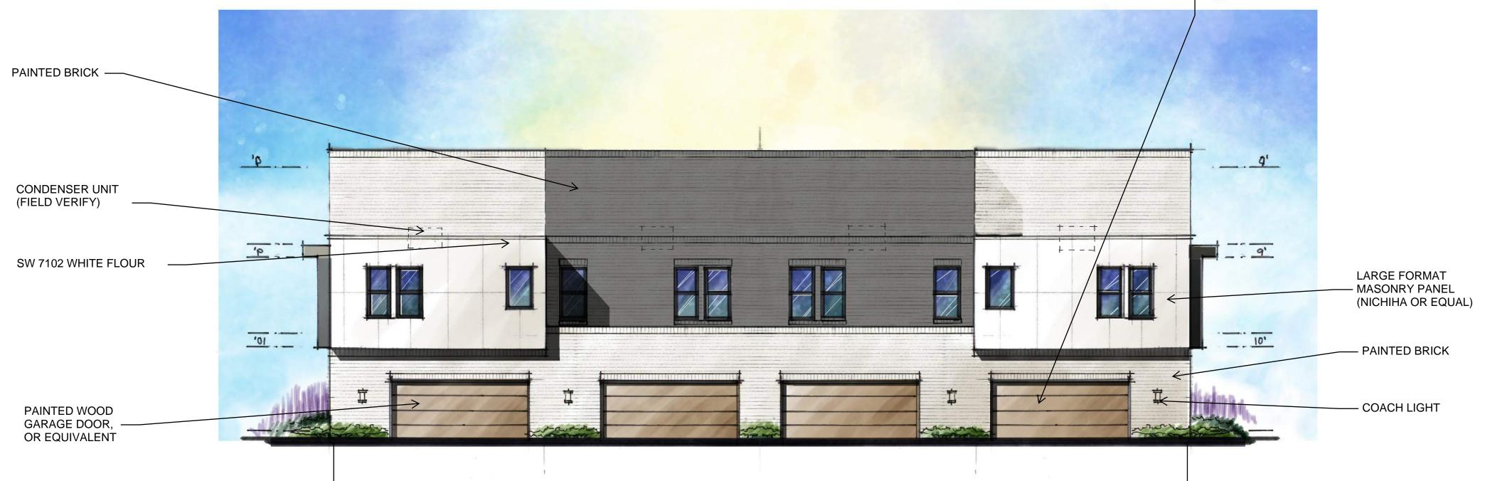
REAR (SOUTH) FACADE: TOTAL MATERIAL SURFACE AREA = 2771 SQ. FT. MASONRY PANEL: 595 SQ. FT. = 21.48% PAINTED BRICK: 2176 SQ. FT. = 78.52%
