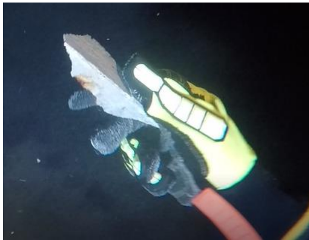
One piece of concrete found on the floor from an edge somewhere in the tank
