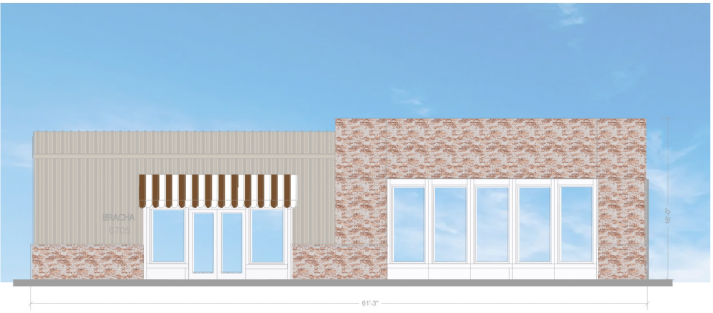
4 BUILDING 2 EAST ELEVATION SCALE: 1/8" = 1'-0"
