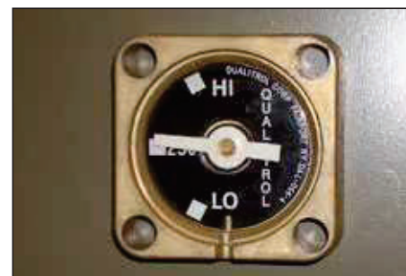
Figure 5. Liquid level gauge.
