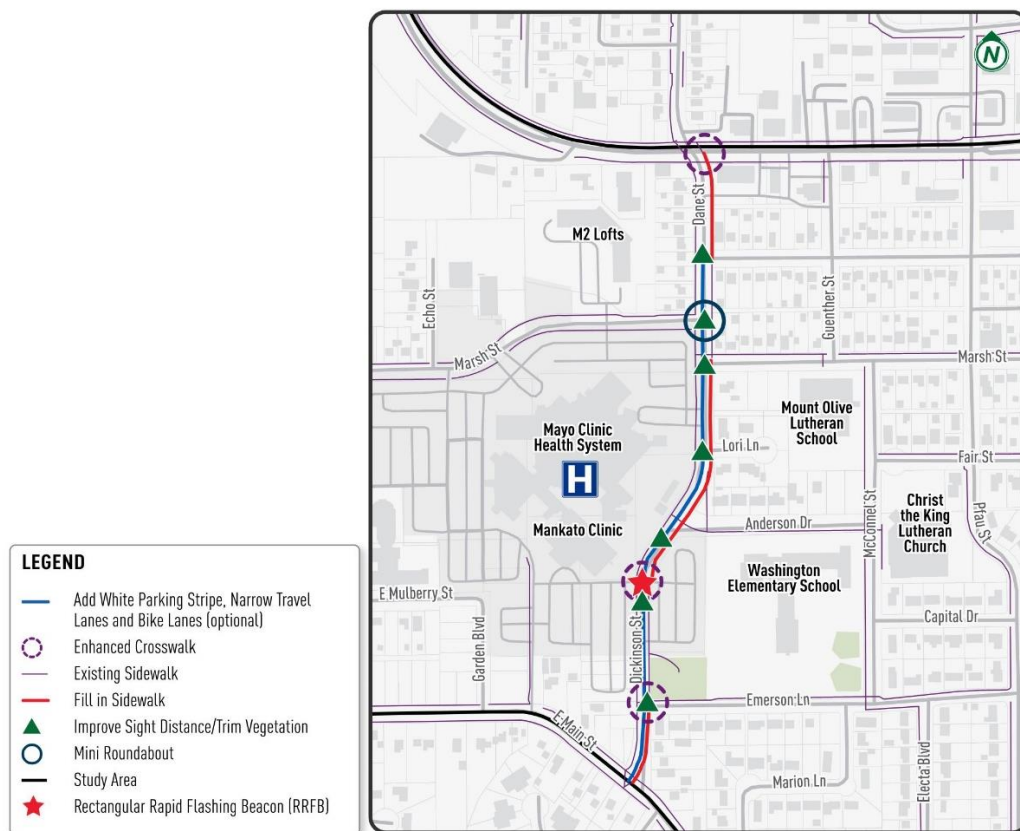
Figure 16. Dickinson St./Dane St. Recommendations
