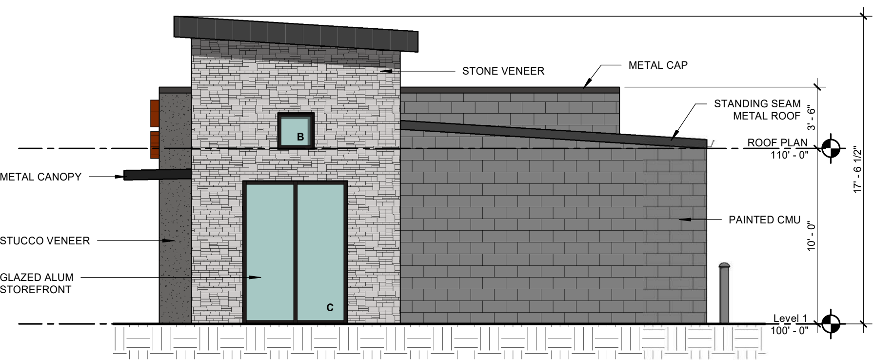
02 BUILDING A EAST ELEVATION 3/16" = 1'-0"
