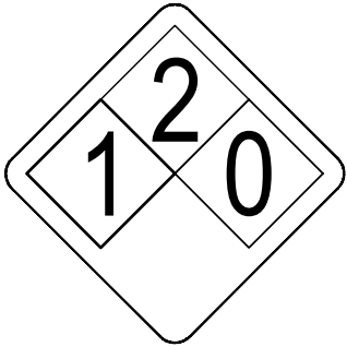
ALERTING SIGN (FOR DIESEL FUEL)
