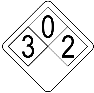
ALERTING SIGN (FOR CELL SITE BATTERIES)
