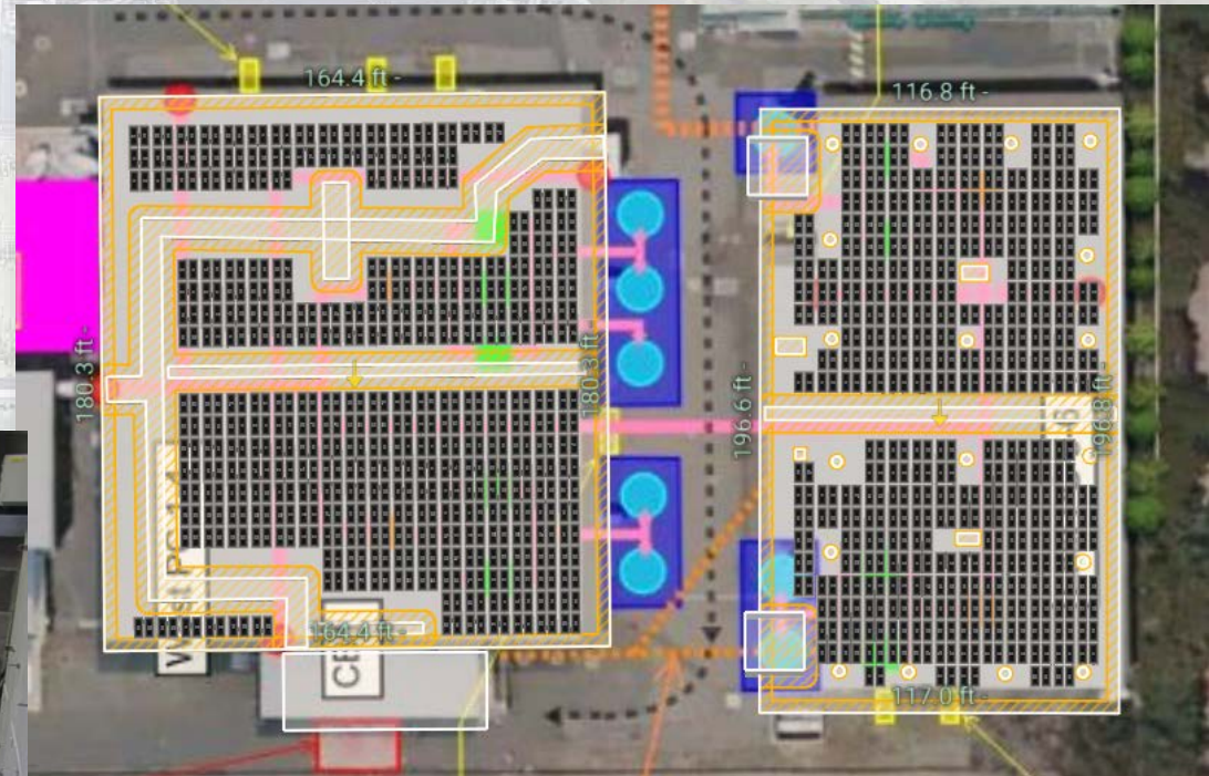
Potential Solar array over Primary Clarifiers at Union City Treatment Plant
