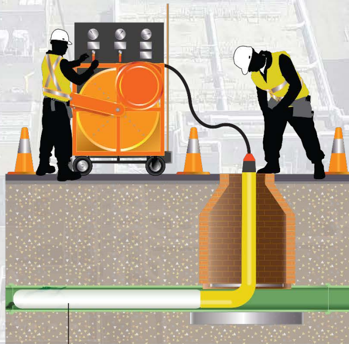
Tube is expanded, resin cures to form a "pipe within a pipe"
