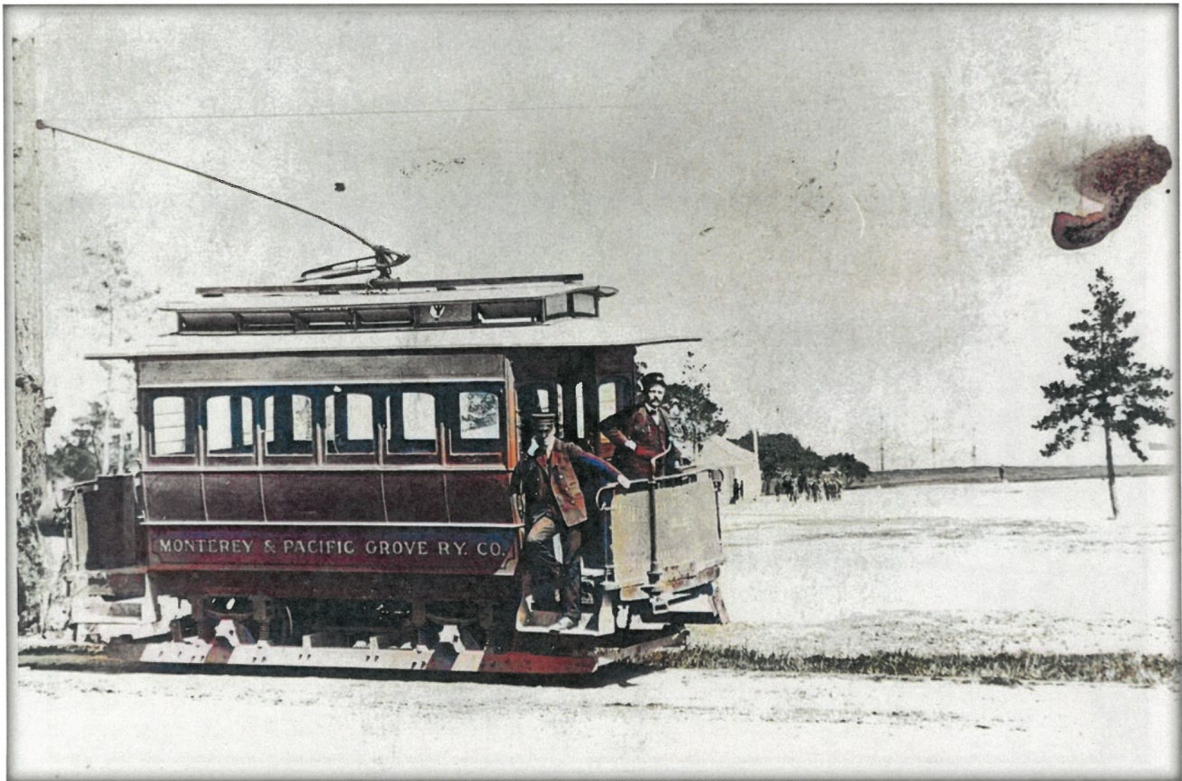
A REBUILT HORSECAR MODIFIED FOR ELECTRIC SERVICE – CIRCA 1905
