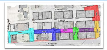
SCOPE: In the work areas defined, replace underground utilities including storm drains, sanitary sewer, and waterlines; demo and replace street surfaces, curbs, and sidewalks; add ramps and handrails to provide safe and accessible pedestrian walkways.
